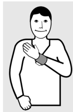
Hold your arm in a relaxed position to your body (see drawing). In this position, your wrist joint with the measuring unit is on a level with your heart.
